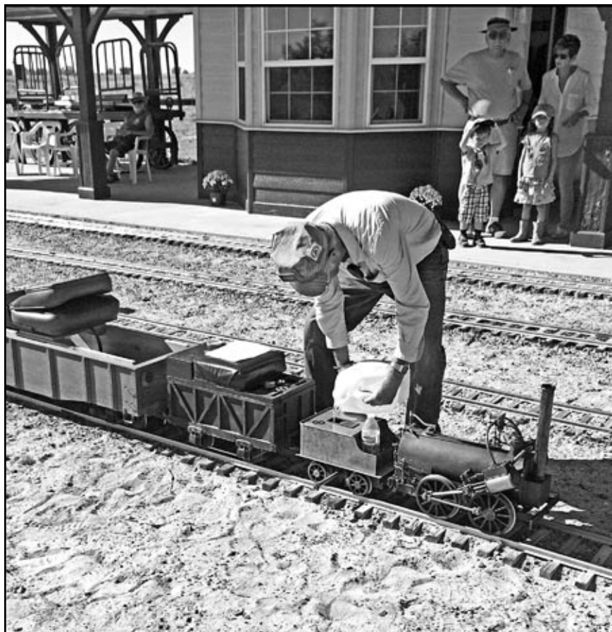
Dean Willoughby watering the tender of “Invicta,” a miniature of the second locomotive built by Stephenson. – Photo © 2018 Steve Mason.
