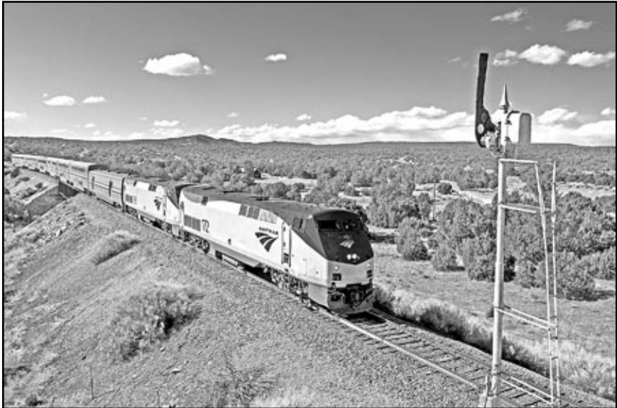
Amtrak 172, P42DC, hustled on time 7-car train 4, the Southwest Chief, past United Switch & Signal Company T-2 style upper quadrant semaphore at the West Siding Switch Chapelle, New Mexico, on March 2, 2020, on BNSF's Glorieta Subdivision. – Photo © 2020 by Chip.
