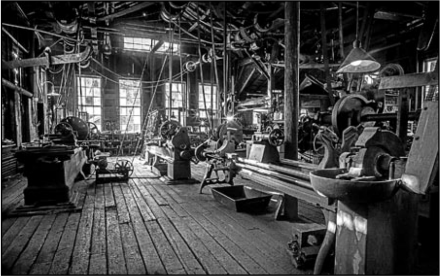
The EBT machine shop in Rockhill, Pennsylvania, on October 8, 2011, completely powered by an overhead belt system. – Photo © 2011 Dennis A. Livesey.
