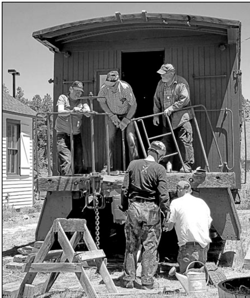
Removing items from the rotted end sill are (from left top) Steve Mason, Jim Scoville, John Rankin, and (from left on ground with backs to camera) John Stephens and Pat Mauro. – Photo © Debbie MacDonald.
