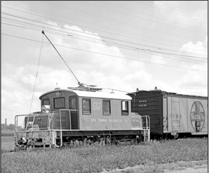
Iowa Traction #52 speeds westbound with three reefers it just picked up from the Mason City interchange. This old Baldwin freight motor has already seen 45 years of service, having begun on the Northeast Oklahoma Railway in 1919. Owned by the Iowa Terminal for only a year at this point, its career will end in a engine house fire only three years later.
