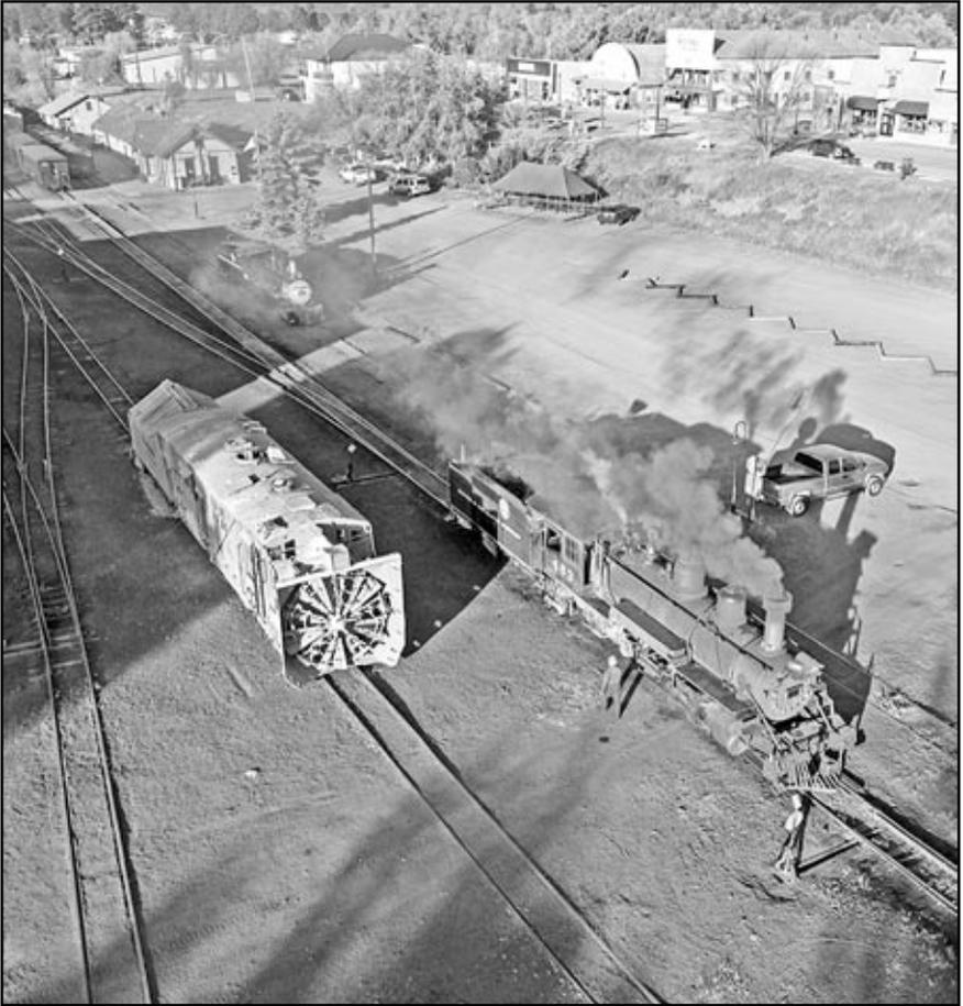
Cumbres & Toltec Scenic RR moved Denver & Rio Grande Western rotary OY (on left, last operated in 1997) from Chama, New Mexico, to Antonito, Colorado, on June 13, 2019. Plans are to prep the OY for limited snow removal in early 2020. Rio Grande 463, a K-27 Mudhen, moved the rotary along with coach 500 – named ALAMOSA and a caboose 0306 from Chama, – Photo © 2019 by Chip.
